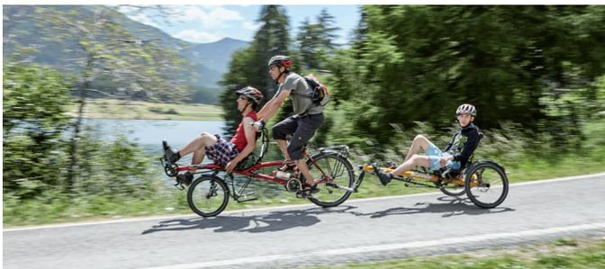
**The trailer set makes it possible to hang the KETTWIESEL and the TRIX behind a normal bicycle like a bicycle trailer.**
