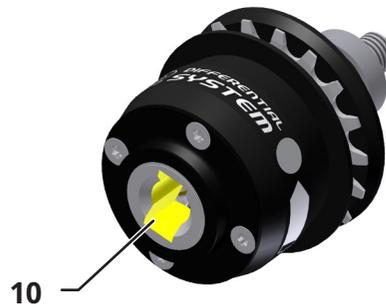
10. Align the differential with the slot nuts. Then slide the left axle assembly as far as it will go into the axle tube. Push the rubber bellows (Ø2) back over the sliding block carrier onto the differential.
